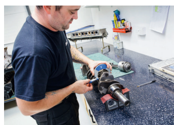
Mark Read checks crank with micrometer
