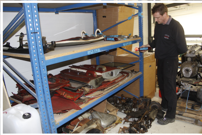
Individual components will be classified as needing refurbishment or replacement, and kept on racking dedicated to that car. To further avoid confusion, parts which need to match the car's body, like the tail lights seen here, are labelled with the job number.
