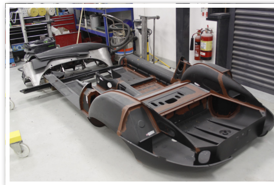
New body parts are ordered as necessary from such as Martin Robey. If the original shell is particularly poor, major elements like the full under-structure may need replacing with a sub-assembly as shown here.
