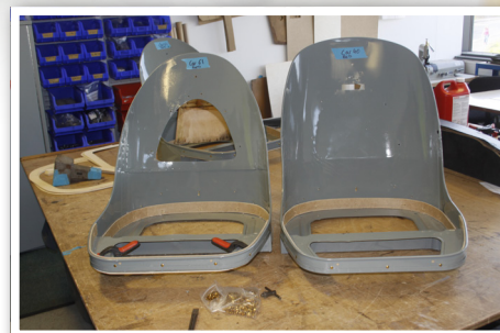
Seats are trimmed from scratch; this is a useful comparison showing the difference between 3.8 litre open two seater (left) and fixed head seats, the latter being markedly broader and taller.
