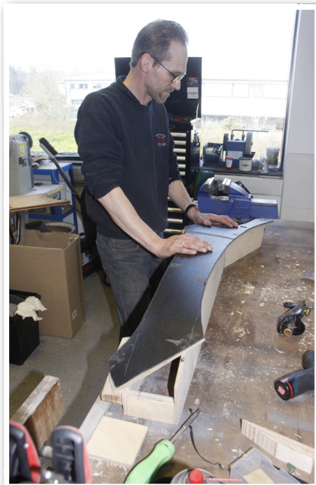
This wooden jig has been made so that the curvature of the card backing will be taken into account when stretching the Vinyl over it.
