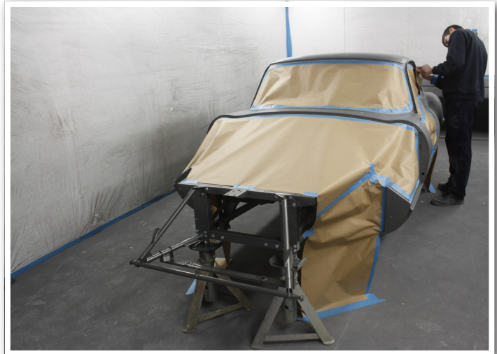
Repaired, the body along with bonnet, doors and trunk lid or hatch are prepared for painting and taken into the in-house paint booth.
