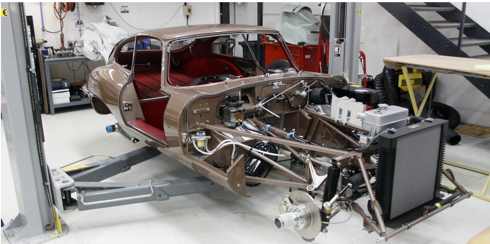
With all major parts restored or replaced, the build up can begin. This is a 3.8 litre car coming together, with a Fosseway radiator in place. This LHD bronze fixed head is to standard specification complete with bellows servo. The detail finish is impressive and experts are consulted on originality issues.
