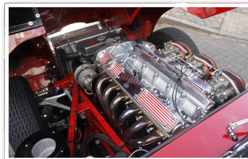
All sorts of upgrades are offered, including 5-speed gearboxes, Weber carburetors and Classicfabs branch exhaust systems as shown here.
