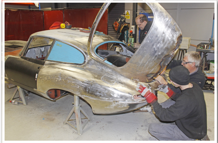
With the body stripped and blasted to remove paint and rust, it goes to the body shop where panels are repaired or replaced.
