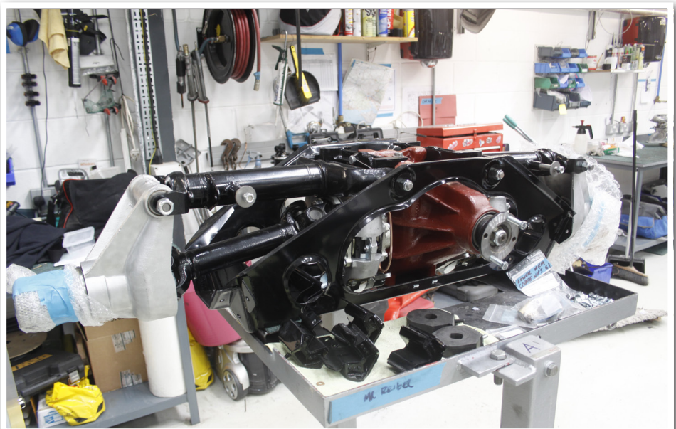
The rear suspension is refurbished and will be offered up to the car as a unit.
