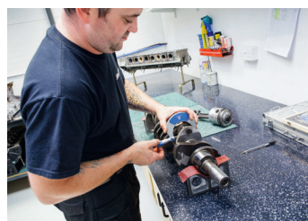
Mark Read checks crank with micrometer
